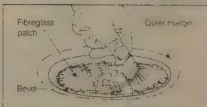
Use plenty of resin when stippling
